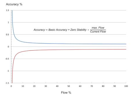
This diagram shows typical values. Individual values may be taken from the calibration records supplied with each meter.
